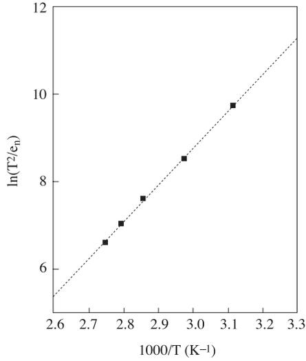
**Figure 4.** Arrhenius plot of the 0.75 eV deep trap observed in GaInP.
