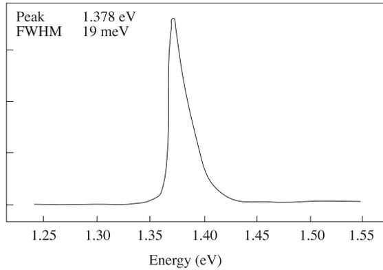
**Figure 2.** Room temperature photoluminescence spectrum for the bulk  $\text{In}_{0.1}\text{Ga}_{0.9}\text{As}$  sample
