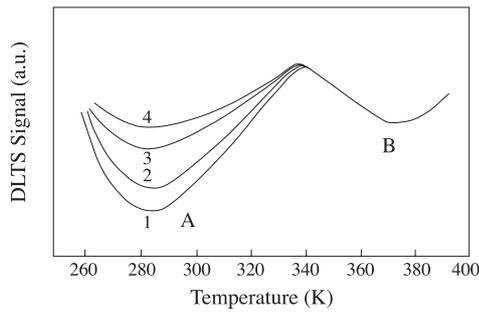
**Figure 6.** DLTS spectrum of a strained GaInP/In<sub>0.15</sub>Ga<sub>0.85</sub>As/GaAs sample with InGaAs channel thickness of 150 Å
