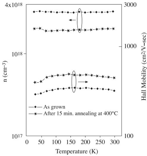
**Figure 3.** Results of the Hall-Effect measurements on the highly doped single GaInP layer (substrate is removed).
