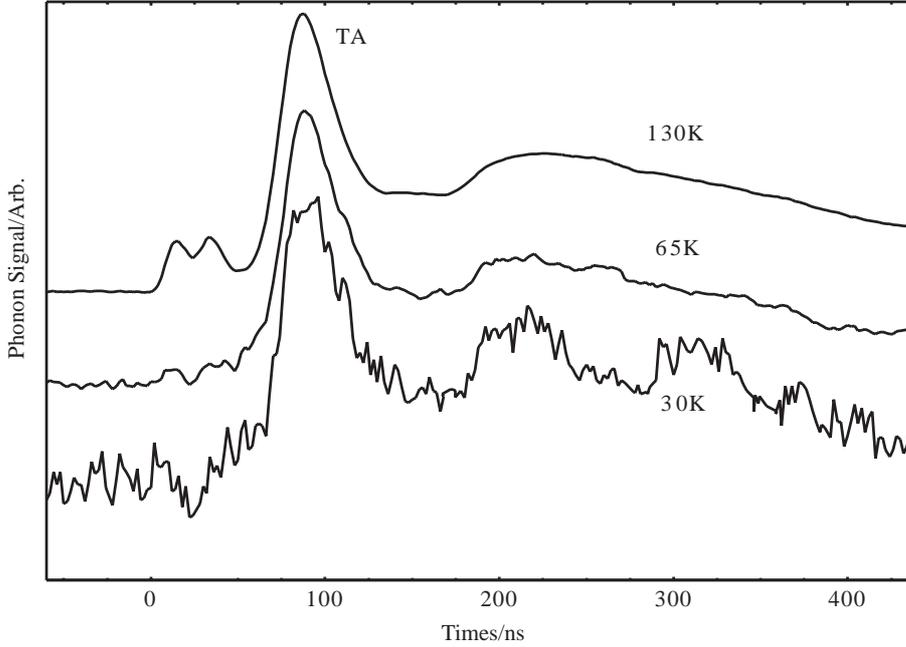
**Figure 4.** Time-of-flight traces for GaN on sapphire sample.
