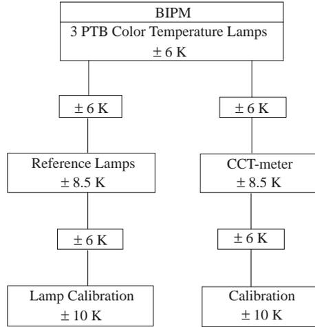
**Figure 1c.** Traceability chain for Color Temperature measurements.
