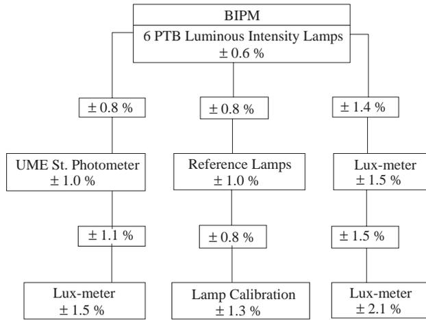
**Figure 1a.** Traceability chain for Luminous Intensity measurements.
