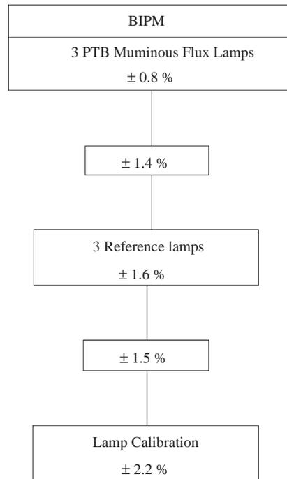
**Figure 1b.** Traceability chain for Luminous Flux measurements.
