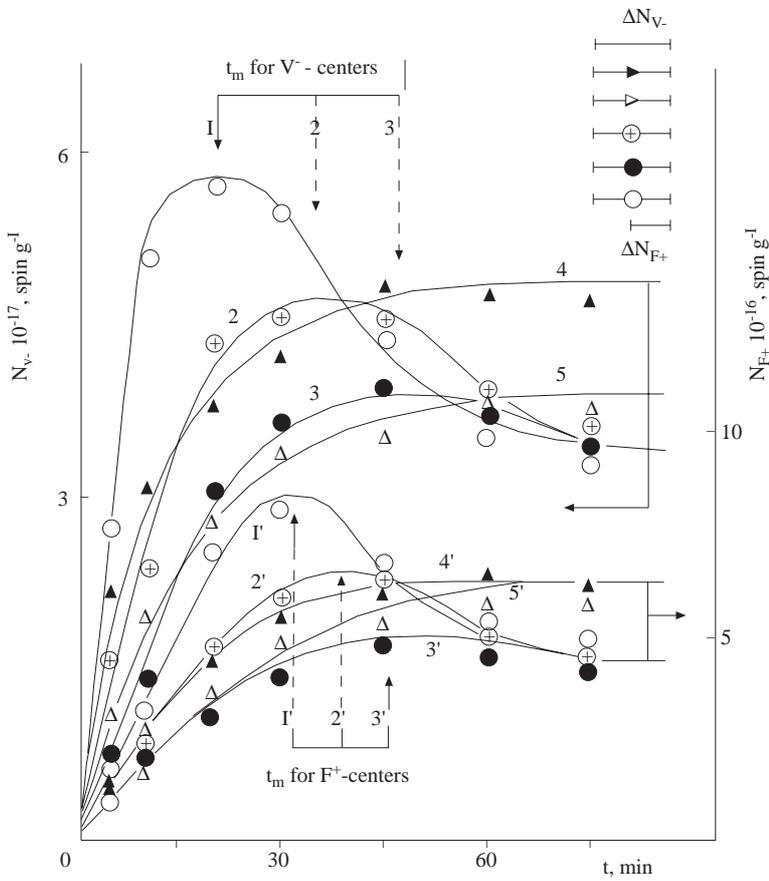
**Figure 2.** The accumulation kinetics of hole  $V^-$  (1-5) and electron  $F^+$  (1'-5')-centers in BeO under electric discharge action in oxygen (1-3 and 1' -3') and in air (4,5 and 4', 5') at 77K;  $E=2.5 \cdot 10^6$  V/m,  $P=1,3$  (curves 1,1');  $1.3 \cdot 10^2$  (2, 2' and 4,4') and  $1.3 \cdot 10^4$  (3,3' and 5, 5') Pa
