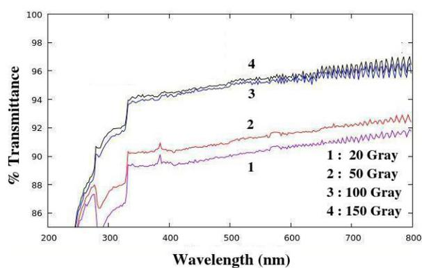
**Figure 1.** UV-Vis transmission spectra of the gamma irradiated specimens.
