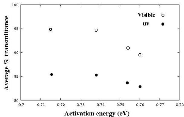
**Figure 2.** Average transmittance vs. activation energy for Pokalon.
