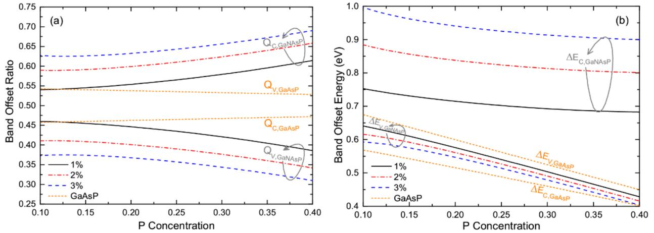
**Figure 1.** Variation in (a) band offset ratio of  $Q_c$  and  $Q_v$  and (b) band offset energies of  $\Delta E_c$  and  $\Delta E_v$  in  $\text{GaN}_x\text{As}_{1-x-y}\text{P}_y/\text{GaP}$  QW on Si substrate as a function of phosphide and nitrogen concentration.
