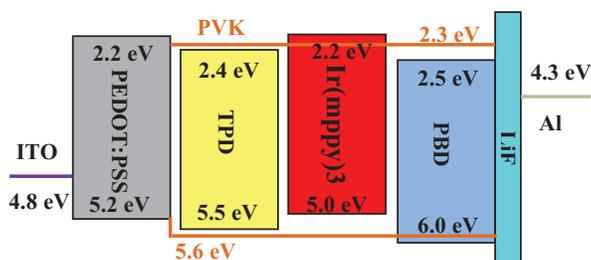
Figure 2. The energy diagram of the device.
