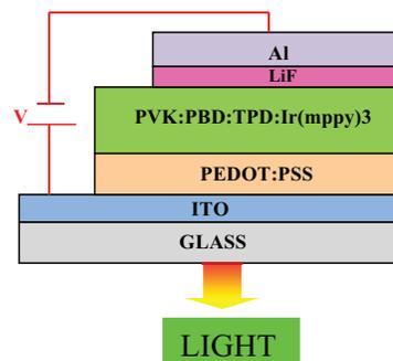
Figure 3. The structure of the device.
