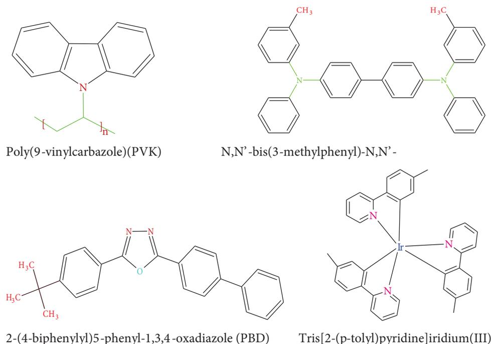
**Figure 1.** The molecular structure of active layer materials.
