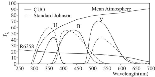
**Figure 2.** Transmission curves of UVB Optec™ filters (continuous lines), transmission curves of standard Johnson UVB filters (from [10]) (dashed line), response curve of Hamamatsu R6358 photocathode in SSP5A model photometer (continuous lines) used at ÇUO and transmission curve of atmospheric transparency (continuous lines) (from [11]).
