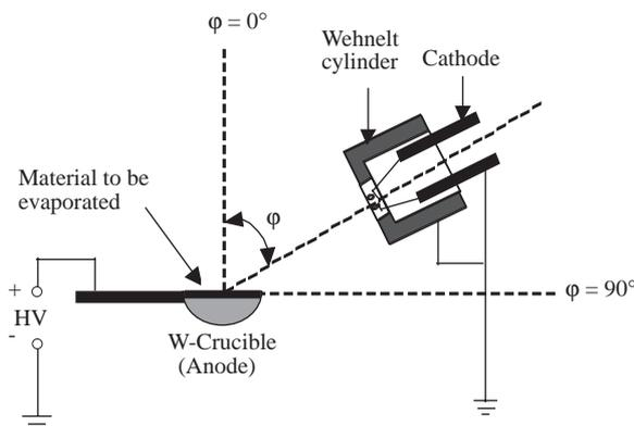
**Figure 1.** Schematic diagram of the TVA electrodes arrangement for  $\varphi > 0^\circ$ . The electrodes (cathode and anode) can be arranged in various relative angular positions  $\varphi$  and distances  $d$  to the anode.  $d$  is the distance between the front surface of the Wehnelt cylinder and the end side of the crucible for the case  $\varphi = 90^\circ$ . The notation HV indicates the high voltage power supply.
