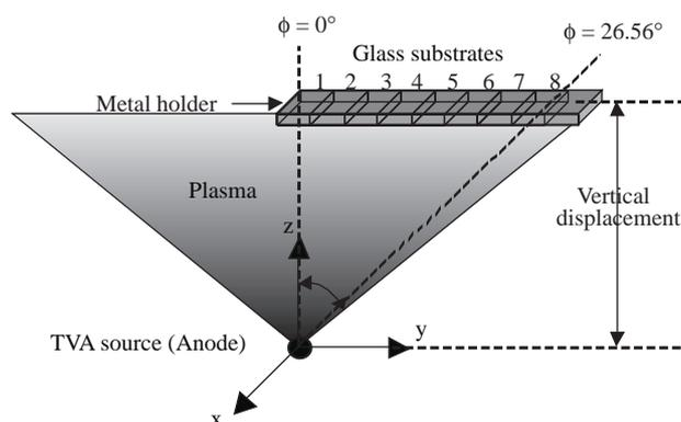
**Figure 3.** Experimental arrangement for the deposition on glass substrates at various angles and distances with respect to the TVA source (anode).
