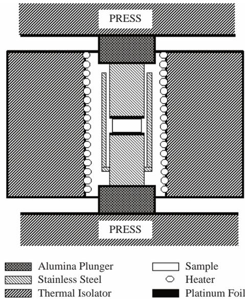
Figure 1. Schematic diagram of the hot-pressing equipment.
