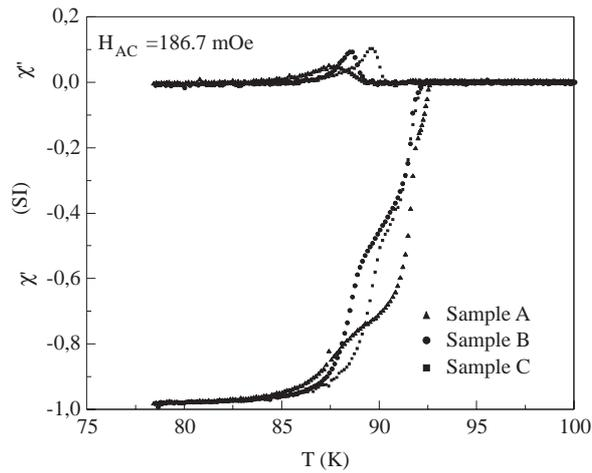
**Figure 4.** AC susceptibility versus temperature variation of the samples A,B and C at 186.7 mOe magnetic field.
