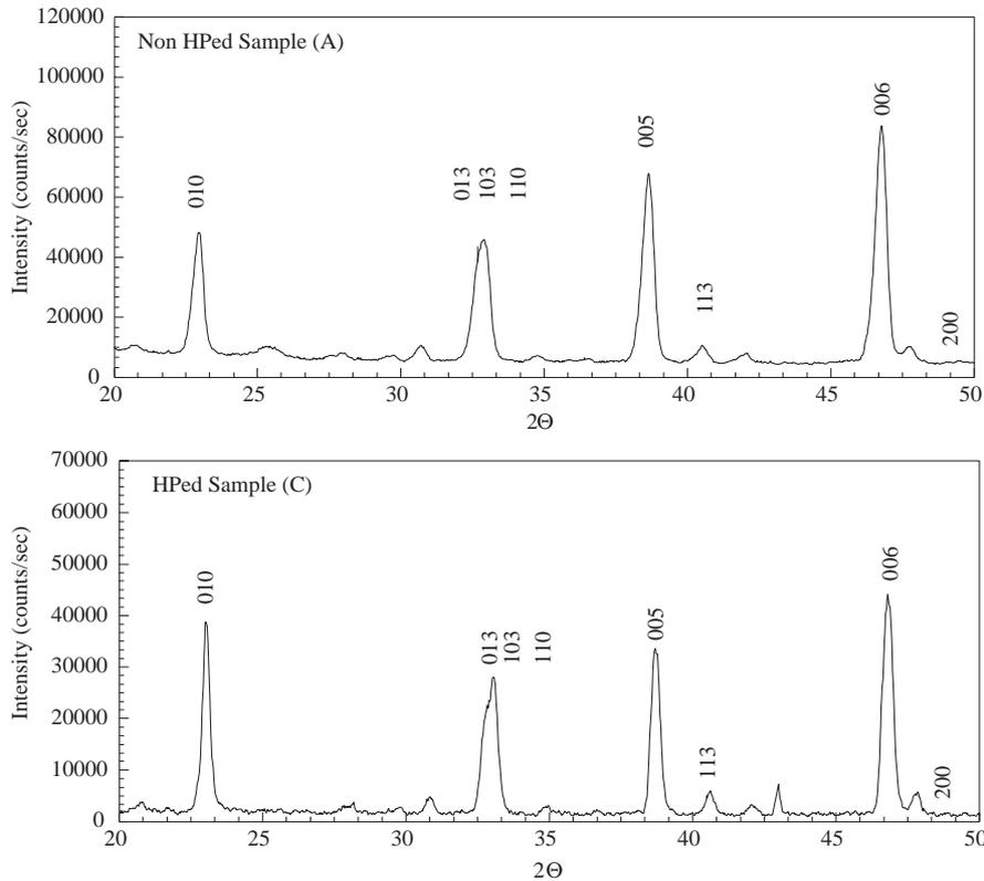
**Figure 2.** XRD patterns of non HPed and HPed sample C.
