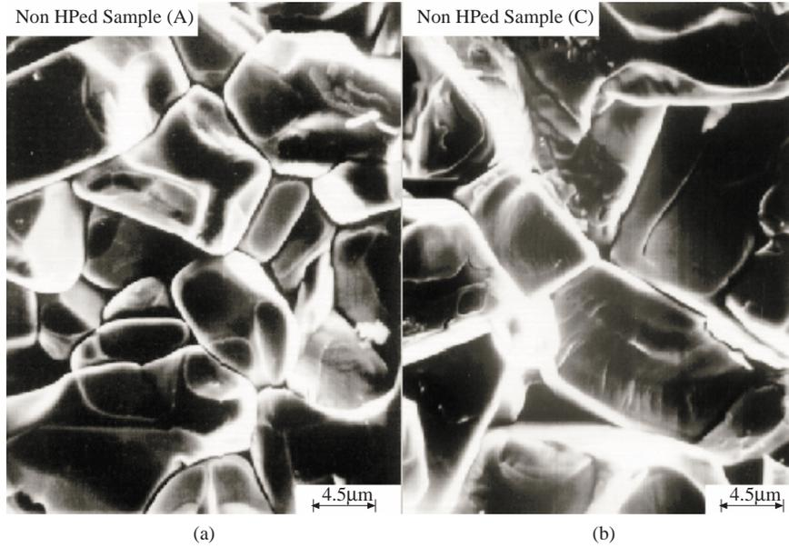
**Figure 3.** SEM images for YBCO (a) non HPed and (b) HPed sample C.
