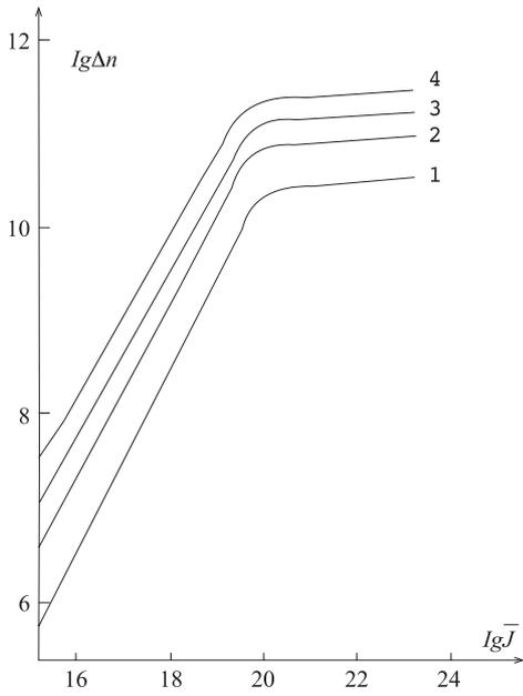
**Figure 2.** Logarithm  $\Delta n$  dependence on illumination  $J$  intensity under the different values of lighting  $J_o$  ( $quantum/cm^2$ ):
