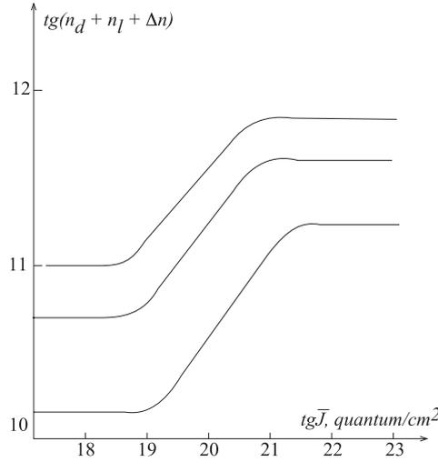
**Figure 3.** Dependence of total electrons concentration in the conductivity zone against illumination intensity under different values of lighting  $J_o$  ( $quantum/cm^2$ ):
