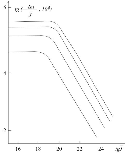
**Figure 5.** Dependence of photoresponce amper - watt sensibility  $(\Delta n/J)$  on  $J$  under different  $J_o(\text{quantum}/\text{cm}^2)$ : 1 -  $10^{16}$ , 2 -  $4 \cdot 10^{16}$ , 3 -  $8 \cdot 10^{16}$ , 4 -  $1.2 \cdot 10^{17}$ .
