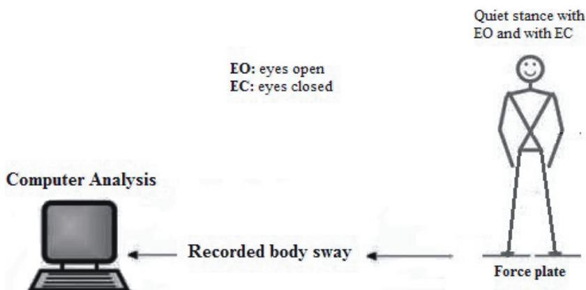
Figure. Schematic image of postural stability measurement.
