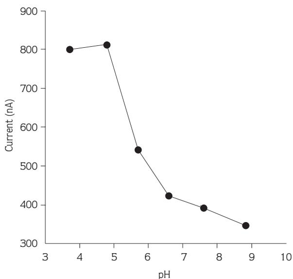
Figure 3. Dependence of the 100  $\mu$ M  $H_2O_2$  response on the solution pH. Batch experiment, stirring the solution at 200 rpm and -0.1 V operating potential in 0.5 M acetate buffer.
