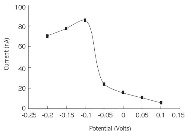
Figure 2. Hydrodynamic voltammogram for 100  $\mu$ M  $\text{H}_2\text{O}_2$  at the HRP-modified CPE. Batch experiment, stirring the solution at 200 rpm in 0.5 M acetate buffer (pH 4.8).
