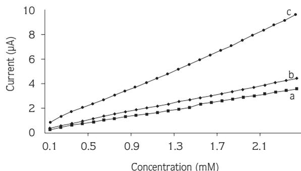
Figure 4. Effect of HRP content in the carbon paste on the hydrogen peroxide response. HRP loadings 2.5 (a), 5.0 (b), 10.0 (c) % (w/w) for carbon paste with 100  $\mu$ M  $H_2O_2$  increments. Other conditions as in Figure 2.
