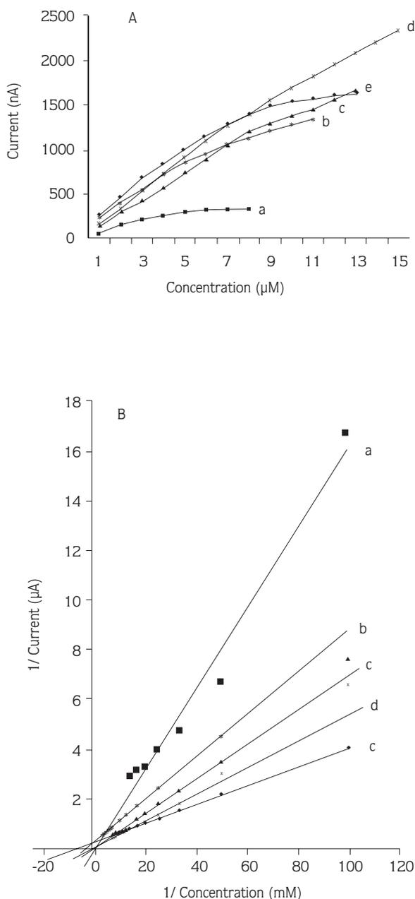
Figure 5. Dependence at the steady state current on the concentration of (a) resorcinol, (b) epinephrine (c) pyrogallol, (d) acetaminophen and (e) pyrocatechol (A)  $i$  vs.  $C$ ; (B)  $1/i_{ss}$  vs.  $1/C$ . Other conditions as in Figure 2.
