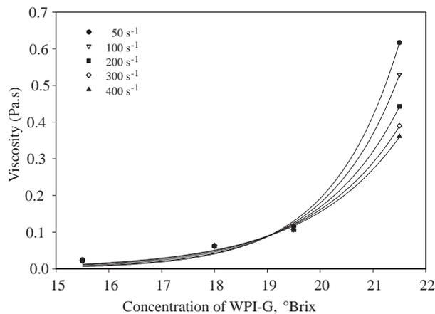
**Figure 5.** Effect of concentration (°Brix) on apparent viscosity of WPI-G solutions at 20°C and different shear rates.
