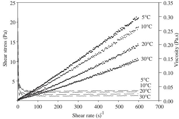
**Figure 1.** Viscosity (lines) and shear stress (symbols) of 15.5° Brix WPI-G solution at different temperatures.
