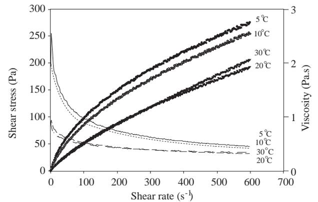
**Figure 4.** Viscosity (lines) and shear stress (symbols) of 21.5° Brix WPI-G solution at different temperatures.
