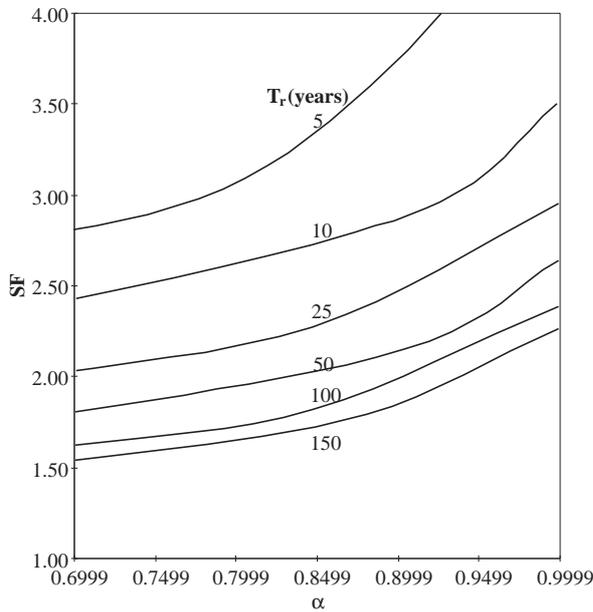
**Figure 4.** Relationship between reliability and safety factor under various return periods for rectangular piers
