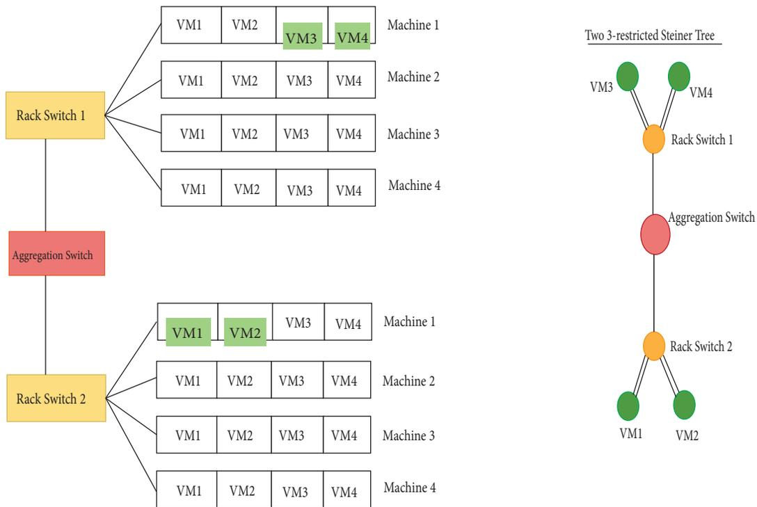
Figure 2. Steiner tree for VDC distribution.
