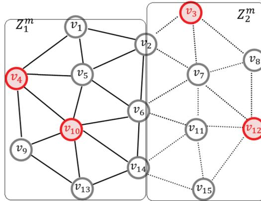
**Figure 3.** An example of network partitioning that fails to accept multicast session  $m$ , where  $s_m = v_4$  and  $R_m = \{v_3, v_{10}, v_{12}\}$ .
