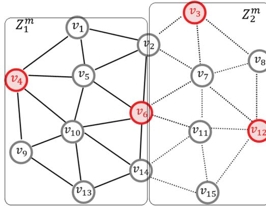
**Figure 1.** Network partitioning to investigate the acceptance of multicast session  $m$ , where  $s_m$  and  $R_m$  are equal to  $v_4$  and  $\{v_3, v_6, v_{12}\}$ , respectively. The links of each zone are illustrated in a different style.
