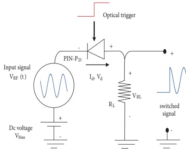
**Figure 1.** Basic PIN-PD-based sampling circuit.
