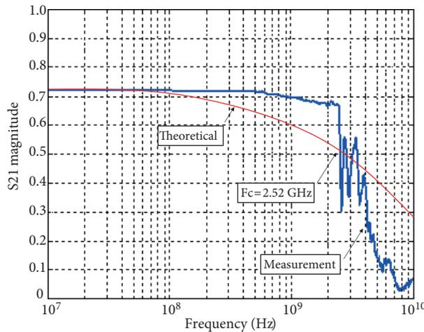
**Figure 7.** Frequency response of the sampling circuit with two demultiplexing stages.
