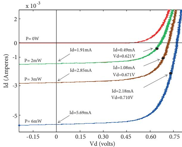
Figure 3. Measured I–V curve of an optically triggered switch based on an InGaAs PIN-PD, with  $I_{sat} = 20$  nA,  $R = 0.95$  A/W at  $\lambda = 1550$  nm, and different optical peak power.
