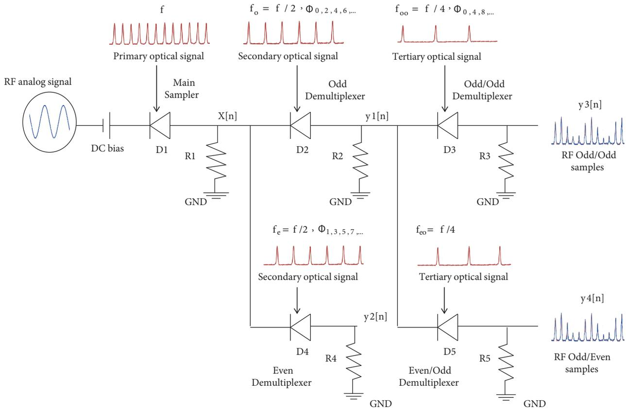
Figure 2. Schematic circuit of the optoelectronic sampling and demultiplexing circuit.
