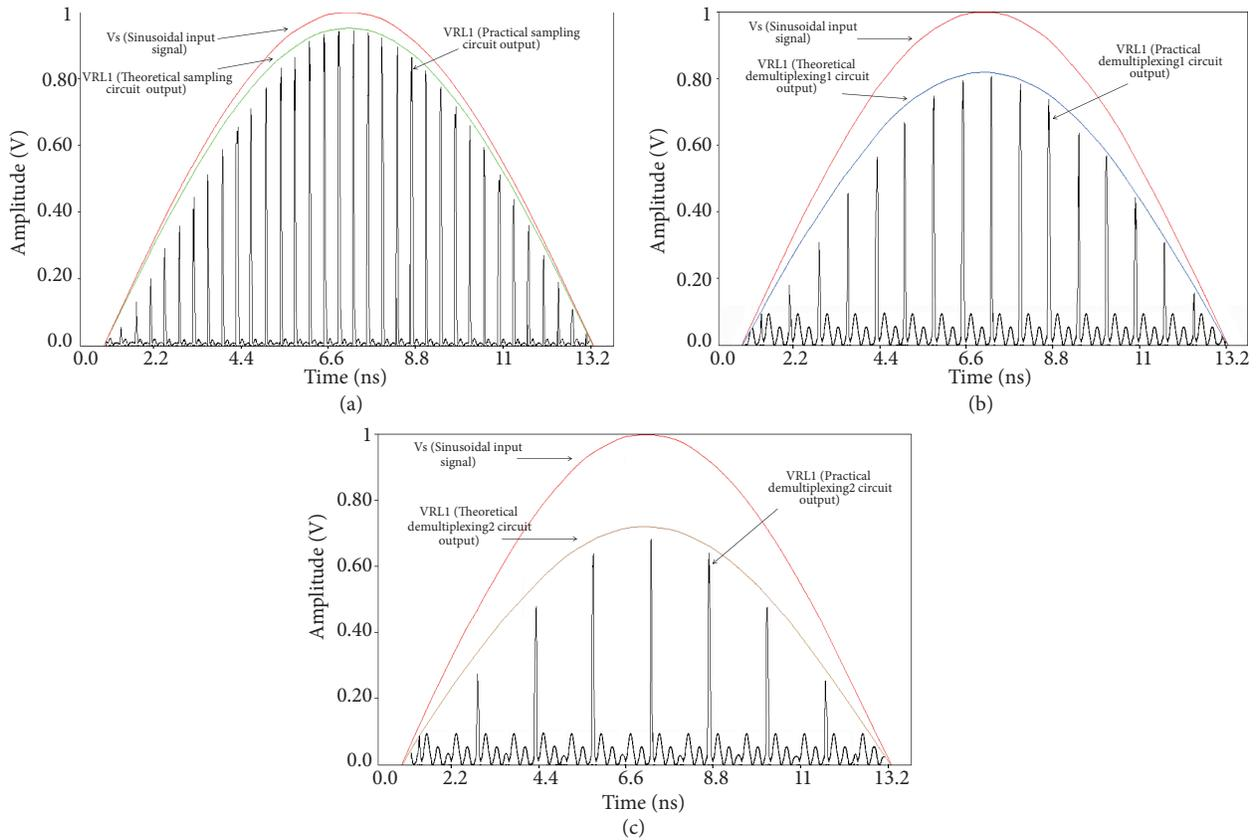
**Figure 6.** Measured outputs of the practical implemented circuit compared to the simulated transient response curves (40 MHz 300 mV peak sinusoidal input signal): a) outputs of the sampling circuit (2.5 GSPS), b) outputs of the first demultiplexing circuit (1.25 GSPS), c) outputs of the second demultiplexing circuit (625 MSPS).
