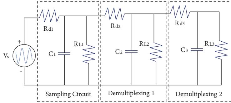
**Figure 4.** Circuit to compute the transfer function of the sampling circuit in cascade connection with two demultiplexing stages.
