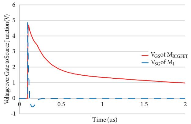
**Figure 8.**  $V_{GS}$  voltage of both transistors under 4 kV ESD shock.
