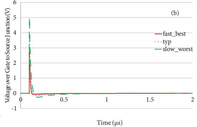
**Figure 9.**  $V_{GS}$  voltage of (a)  $M_{BIGFET}$  and (b)  $M_1$  under 4-kV ESD shock over corner and temperature.
