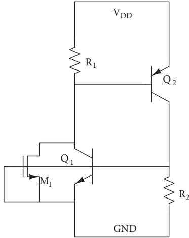
**Figure 2.** Silicon-controlled rectifier.
