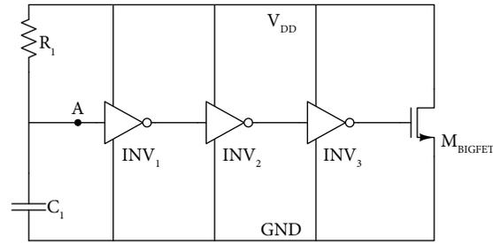
**Figure 3.** A typical RC-triggered ESD power clamp.
