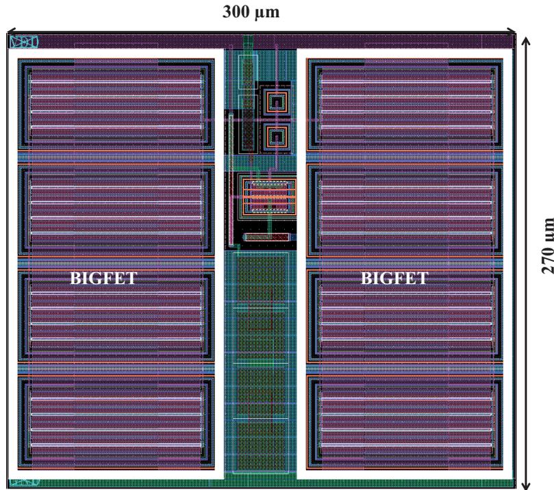
Figure 11. Layout of the ESD clamp.
