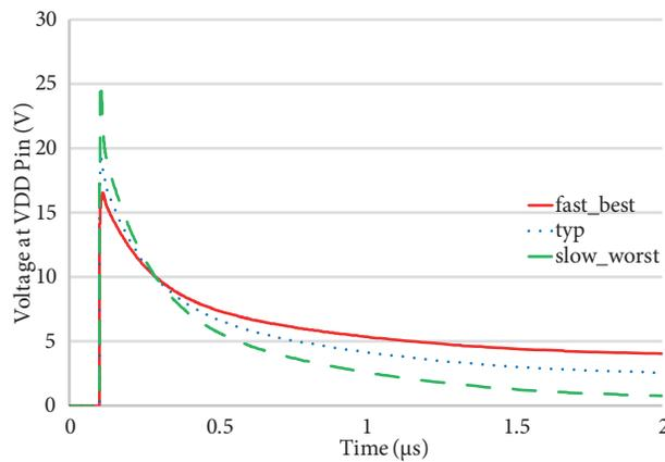
**Figure 10.** Voltage waveforms of the supply pin under 4-kV ESD shock over corner and temperature.
