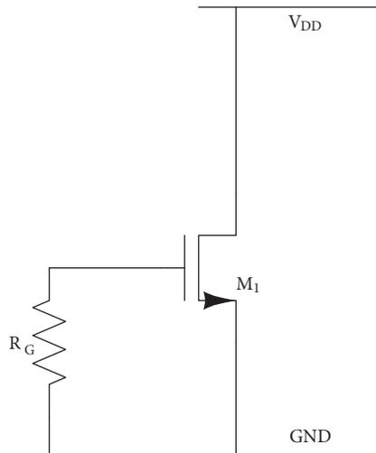
**Figure 1.** Gate-grounded ESD power clamp.
