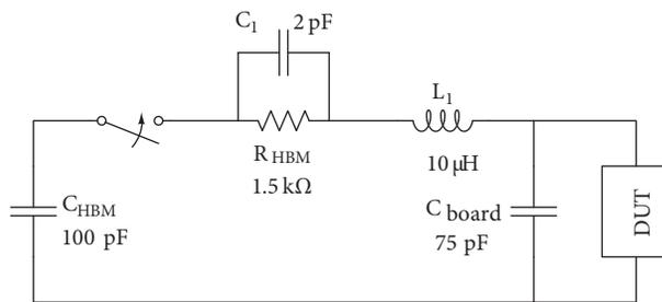
**Figure 6.** Fourth-order human body model ESD simulation bench.
