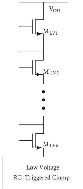
**Figure 4.** HV RC-triggered ESD protection with LV devices.
