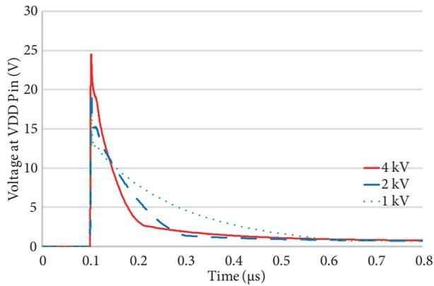
**Figure 7.** Voltage waveforms of the supply pin at various ESD levels.
