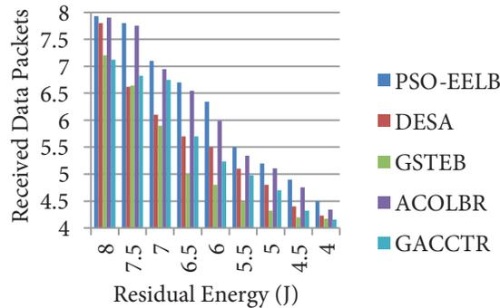
Figure 6. Received data packets versus residual energy.
