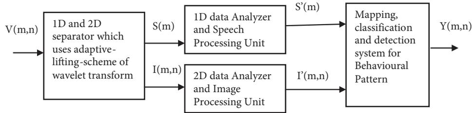
**Figure 1.** Schematic diagram of detection and authentication system.
