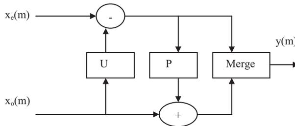
**Figure 3.** The 1D merger using adaptive inverse lifting scheme of wavelet transform.
