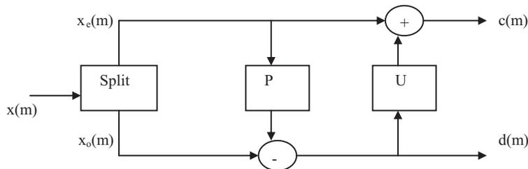
**Figure 2.** The 1D separator using the adaptive-lifting scheme of wavelet transform.
