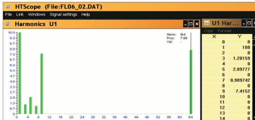
Figure 6. Voltage THD levels for the compensated system.
