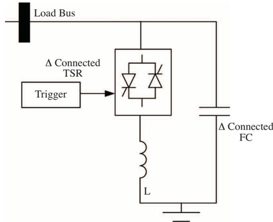
**Figure 1.** TSR-based SVC configuration.
