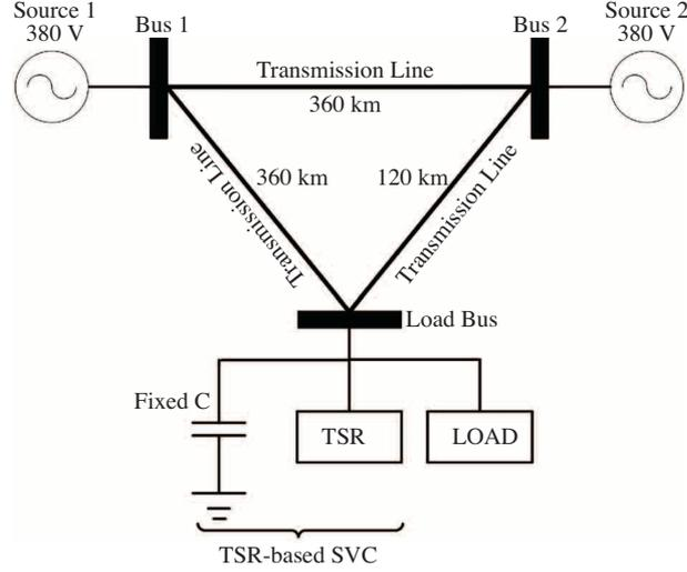
**Figure 2.** One-line diagram of the three-bus system with TSR-based SVC.
