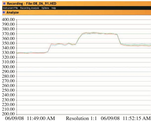
**Figure 9.** Load voltages for the system with the SMIB.
