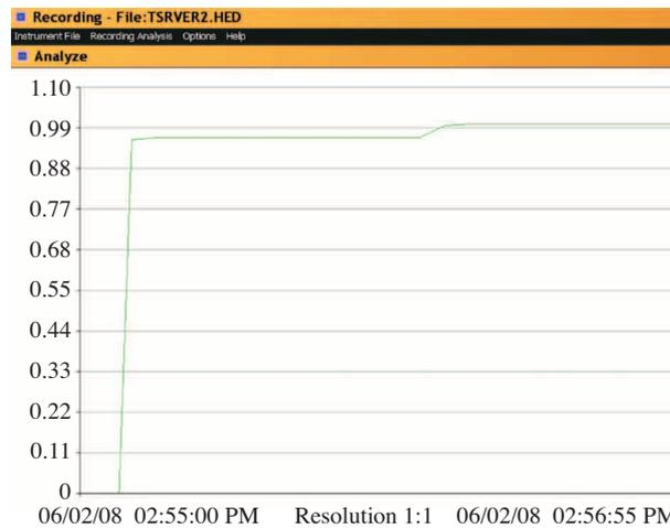
Figure 7. Power factor graphic for the system with TSR-based SVC.
