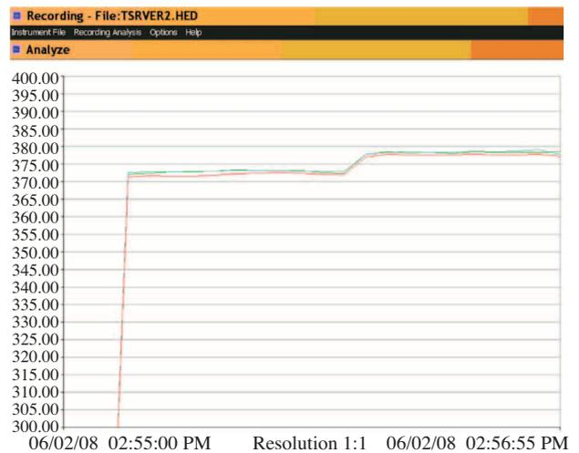
Figure 4. Load voltages in the three-bus system with a TSR-based SVC.
