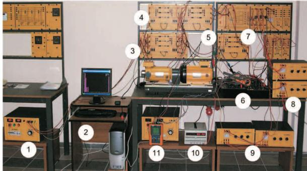
Figure 3. The practical system with TSR-based SVC.
