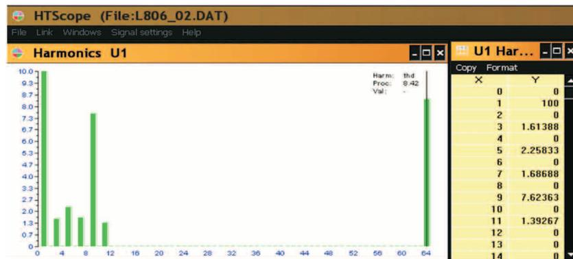
Figure 5. Voltage THD levels for the uncompensated system.
