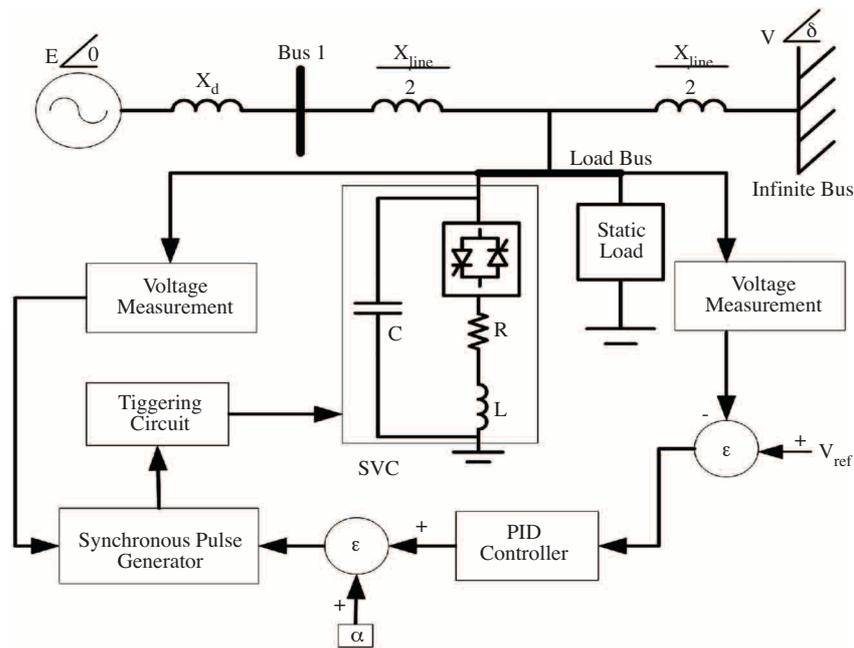
**Figure 8.** One-line diagram of the system with the SMIB.
