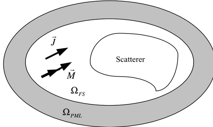
**Figure 4.** A conformal PML configuration.
