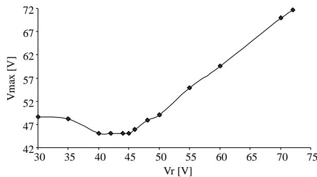
**Figure 10.** Maximum rail voltage vs. voltage threshold of RPCDs ( $V_r$ ) for  $R_G = 0.08 \Omega$ .
