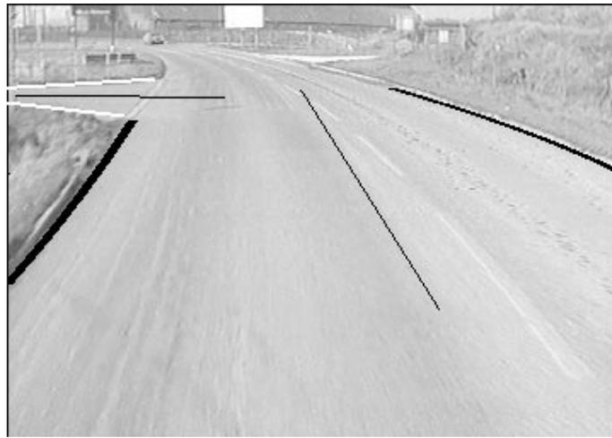
**Figure 11.** Results of edge segments process using edge detector.
