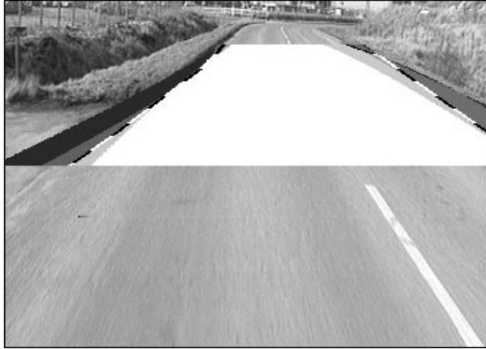
**Figure 2.** Pixel Voting Result. The different grey levels within the voting band of the Pixel-Based Fusion show the strength of belief that that a pixel is in the road. The final road edges displayed on the image are obtained by thresholding the voting space.
