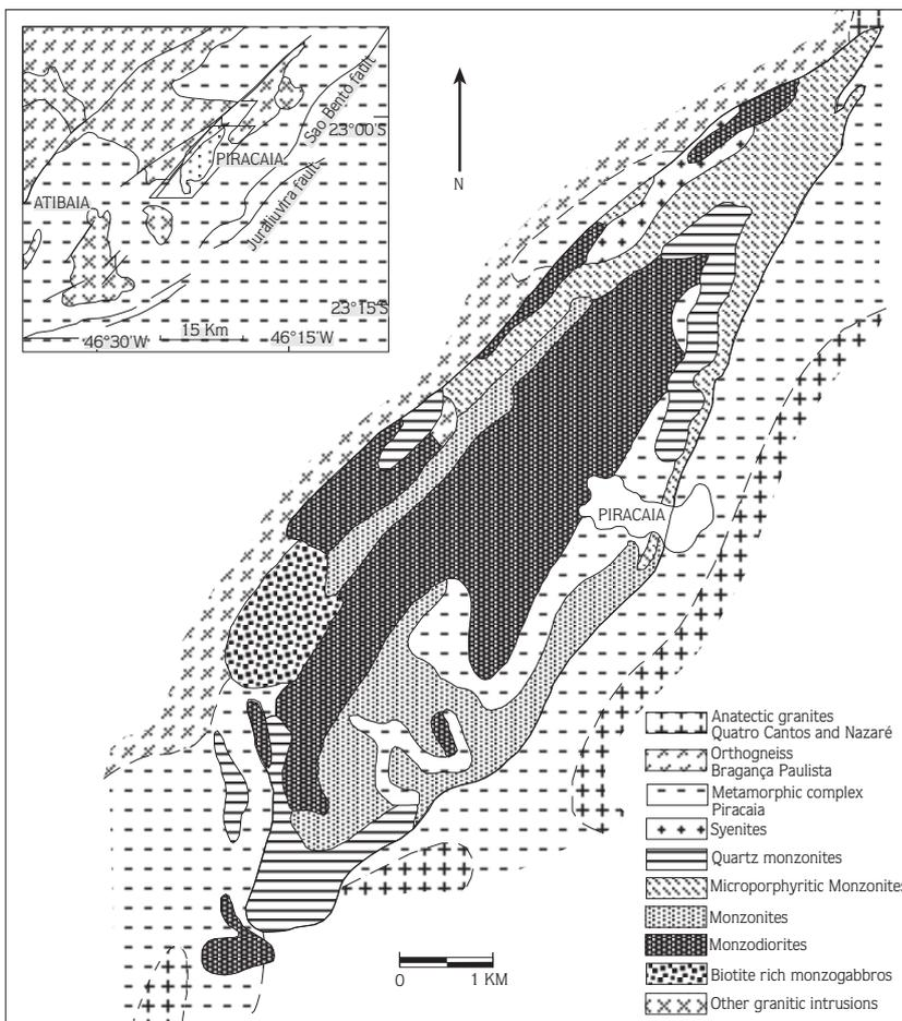
Figure 9. Geological map of the composite complex of Piracaia (after Janasi and Ulbrich, 1987).
