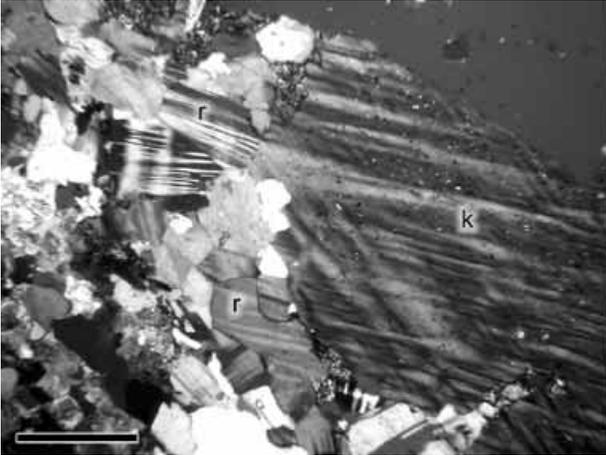
Figure 9. Coarsely recrystallized K-feldspar (r) in the strain shadow of feldspar porphyroclasts (k). Crossed polarizers; scale bar – 0.3 mm.
