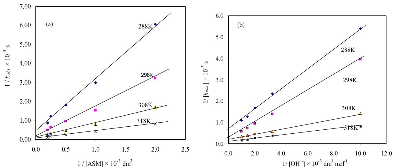
**Figure 2.** (a) Plots of  $k_{obs}$  versus  $[ASM]$  and  $1/k_{obs}$  versus  $1/[ASM]$  and (b)  $k_{obs}$  versus  $[OH^-]$  and  $1/k_{obs}$  versus  $1/[OH^-]$  at 4 different temperatures (conditions as in Table 1).
