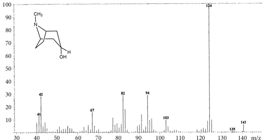
**Figure 5.** GC-MS spectra of tropine showed molecular ion peak at m/z 141 amu and base peak at m/z 124 amu.
