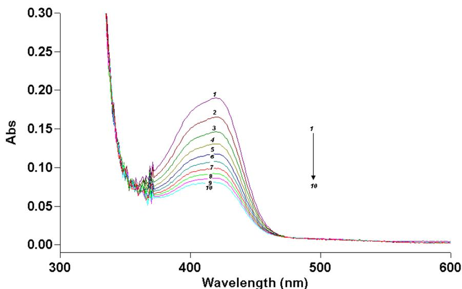
**Figure 3.** UV-Vis spectral changes during the oxidation of atropine sulfate by alkaline hexacyanoferrate(III) at 25 °C;  $[Fe(CN)_6^{3-}] = 2.0 \times 10^{-4}$ ;  $[ASM] = 2.0 \times 10^{-3}$ ;  $[OH^-] = 0.5$ ; and  $I = 1.0 \text{ mol dm}^{-3}$  with scanning time interval of 1.0 min.
