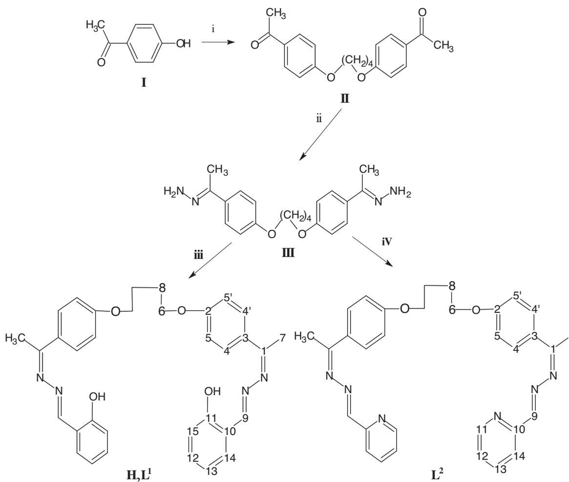
**Scheme. i**,  $\text{Br}-(\text{CH}_2)_4-\text{Br}$  and  $\text{K}_2\text{CO}_3$ , acetone, reflux 15 h; **ii**,  $\text{NH}_2\text{NH}_2 \cdot \text{H}_2\text{O}$ , EtOH, reflux 4 h.; **iii**, salicylaldehyde, EtOH, reflux 4 h.; **iv**, pyridine-2-carbaldehyde, EtOH, room temperature.
