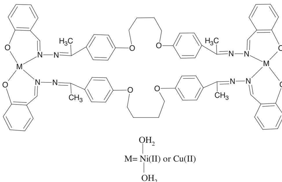
**Figure 3.** Proposed structure of the double-stranded binuclear complexes of  $\text{H}_2\text{L}^1$  [ $\text{M}=\text{Ni(II)}$  or  $\text{Cu(II)}$ ].
