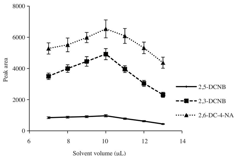
**Figure 2.** Effect of solvent volume on extraction of analytes; Conditions: sample volume 14 mL, analytes concentration  $50 \text{ ng L}^{-1}$ , salt concentration  $1 \text{ mol L}^{-1}$ , sample temperature  $50 \text{ }^\circ\text{C}$ , stirring rate 1000 rpm, extraction time 30 min, each point is the average of 3 independent measurements.
