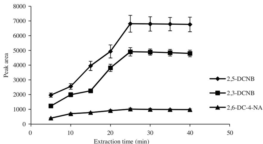
**Figure 4.** Effect of extraction time; Conditions: sample volume 14 mL, analytes concentration  $50 \text{ ng L}^{-1}$ , salt concentration  $1 \text{ mol L}^{-1}$ , sample temperature  $50 \text{ }^\circ\text{C}$ , organic phase volume  $10 \mu\text{L}$ , stirring rate 1000 rpm, each point is the average of 3 independent measurements.
