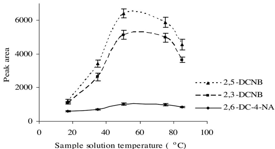
**Figure 3.** Effect of sample temperature extraction of analytes; Conditions: sample volume 14 mL, analytes concentration  $50 \text{ ng L}^{-1}$ , salt concentration  $1 \text{ mol L}^{-1}$ , organic phase volume  $10 \mu\text{L}$ , stirring rate 1000 rpm, extraction time 30 min, each point is the average of 3 independent measurements.
