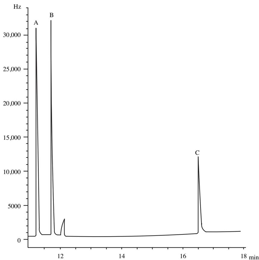
**Figure 1.** Chromatogram of investigated analytes in 1-undecanol under optimum temperature conditions of GC. (A) 2,5-dichloro-nitrobenzene, (B) 2,3-dichloro-nitrobenzene, (C) 2,6-dichloro-4-nitroaniline; Conditions: sample volume 14 mL, analytes concentration  $50 \text{ ng L}^{-1}$ , salt concentration  $1 \text{ mol L}^{-1}$ , sample temperature  $50 \text{ }^\circ\text{C}$ , organic phase volume  $10 \text{ } \mu\text{L}$ , stirring rate 1000 rpm, extraction time 30 min.
