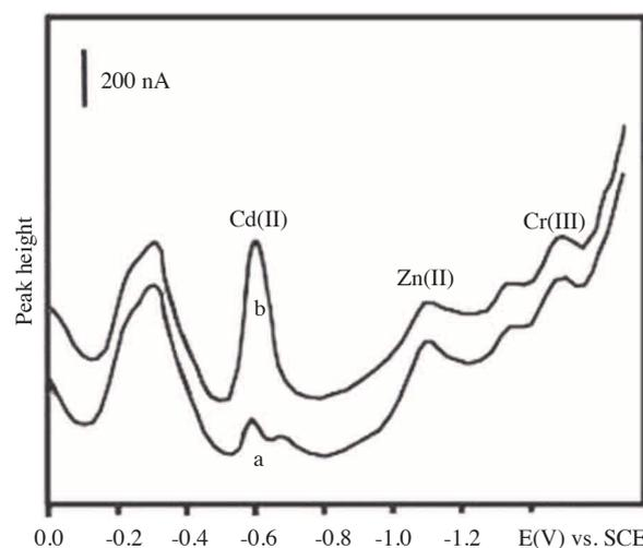
**Figure 4.** Determination of Cd in cow liver pH 8.5 acetate (inhibited interference of Se), (a) 7.0 mL 0.1 M NaAc + 0.1 mL liver sample, (pH 8.5), (b) curve a + 0.1 mL  $1 \times 10^{-3} \text{ M Cd(II)}$ .
