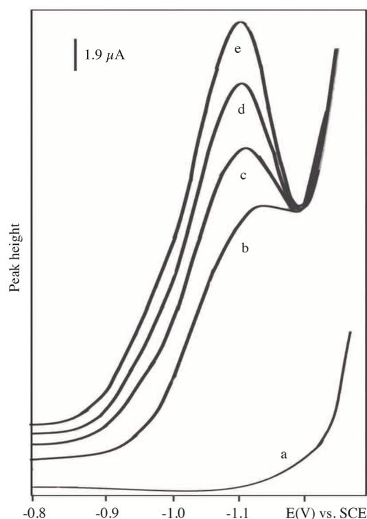
**Figure 9.** Determination of selenium in cow liver by using catalytic peak, (a) 10.0 mL acetate buffer (pH 3.3) + 0.1 mL 100 times diluted cow liver sample, (b) curve a + 0.2 mL  $1 \times 10^{-3}$  M Mo(VI), (c) curve b + 0.3 mL  $1 \times 10^{-4}$  M Se(IV), (d) curve c + 0.3 mL  $1 \times 10^{-4}$  M Se(IV), (e) curve d + 0.3 mL  $1 \times 10^{-4}$  M Se(IV).
