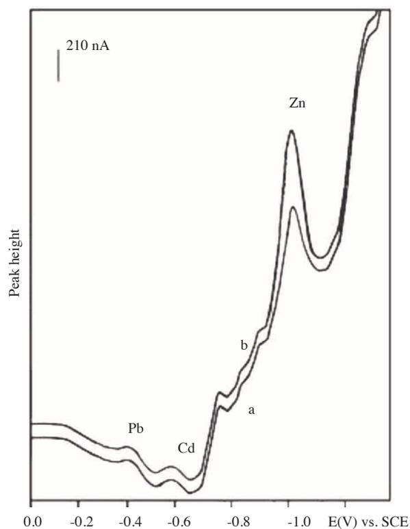
**Figure 8.** Determination of Zn in cow liver using DPP, (a) 10 mL HAc-NaAc + 0.5 mL cow liver sample, (pH 4), (b) curve a + 0.1 mL  $1 \times 10^{-3}$  M Zn(II).
