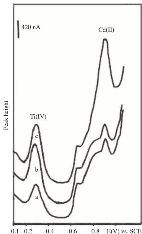
**Figure 3.** Determination of Cd(II) and Ti(IV) in cow liver, (a) 10 mL 0.1 M HAc-NaAc + 1.0 mL 0.1 M EDTA + 0.1 mL liver sample, (pH 4), (b) curve a + 0.1 mL  $1 \times 10^{-3} \text{ M Ti(IV)}$ , (c) curve b + 0.1 mL  $1 \times 10^{-3} \text{ M Cd(II)}$ , (b) curve a + 0.1 mL  $1 \times 10^{-3} \text{ M Cd(II)}$ .
