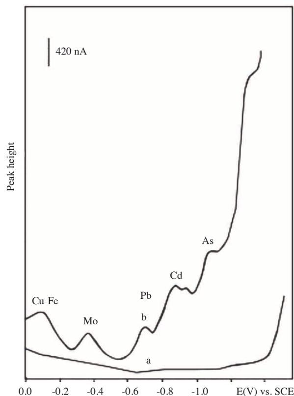
**Figure 1.** DPP polarogram of digested cow liver sample, (a) 10 mL 0.1 M acetate + 1.0 mL 0,1 M EDTA, (pH 2), (b) curve a + 0.1 mL digested liver sample.
