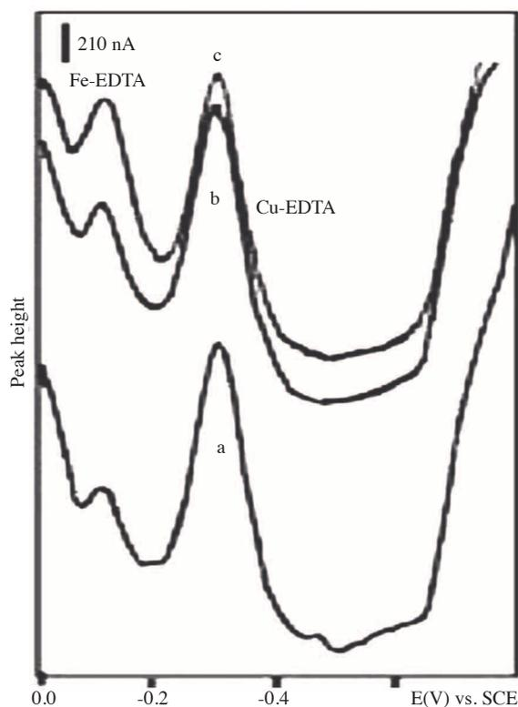
**Figure 7.** Determination of Fe(III) in cow liver pH 5 HAc-NaAc buffer, (a) 8.0 mL HAc-NaAc (pH 5) + 0.1 mL liver sample + 1.5 mL 0.1 M EDTA, (b) curve a + 0.1 mL  $1 \times 10^{-3}$  M Fe(III), (c) curve b + 0.1 mL  $1 \times 10^{-3}$  M Fe(III).
