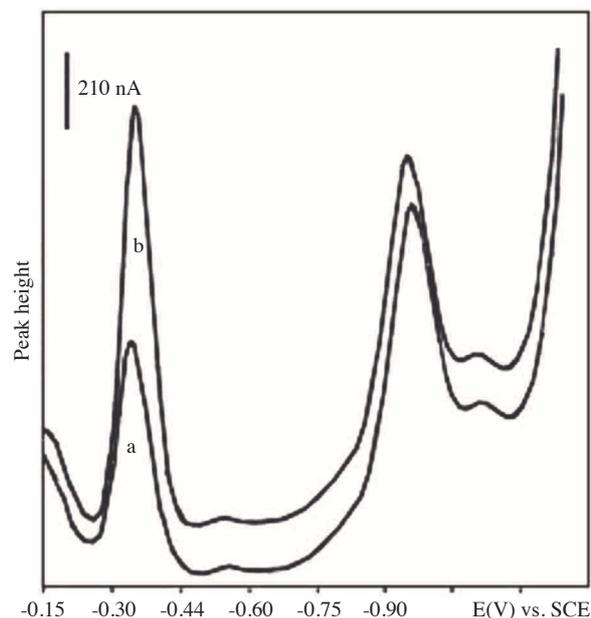
**Figure 6.** Determination of Cu in cow liver pH 8.5 (inhibited interference of Se), (a) 10.0 mL 0.1 M NaAc (pH 8.5) + 1.0 mL liver sample + 1.0 mL 0.1 M EDTA, (b) curve a + 0.1 mL  $1 \times 10^{-3}$  M Cu(II).
