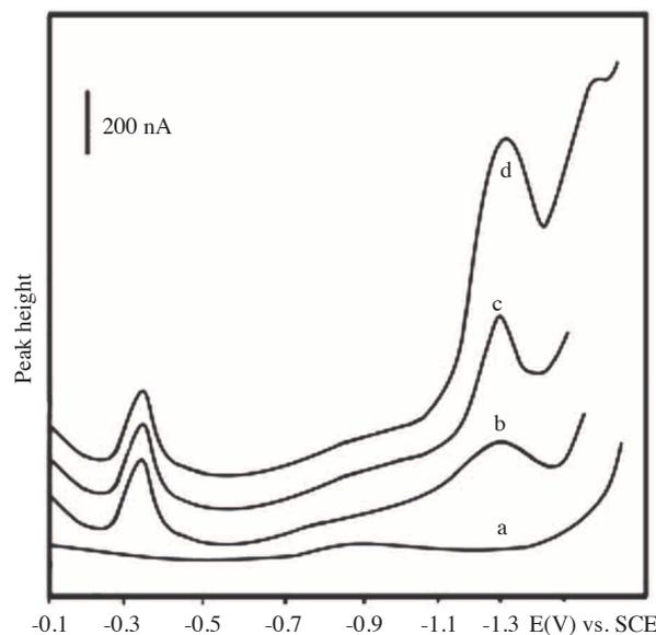
**Figure 2.** Determination of lead in cow liver, pH 8.5 acetate (inhibited interference of Se), (a) 9.0 mL 0.1 M NaAc + 0.1 mL liver sample, (pH 8.5), (b) curve a + 0.2 mL 0.1 M EDTA, (c) curve b + 0.1 mL  $1 \times 10^{-3}$  M Pb(II), (d) curve c + 0.1 mL  $1 \times 10^{-3}$  M Pb(II).
