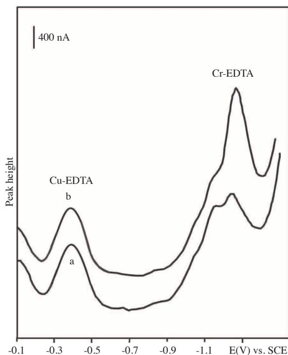
**Figure 5.** Determination of Cr(III) in cow liver sample, (a) 10 mL 0.1 M NaAc + 1 mL 0.1 M EDTA + 0.1 mL liver sample, (pH 6.0), (b) curve a + 0.1 mL  $1 \times 10^{-3}$  M Cr(III).
