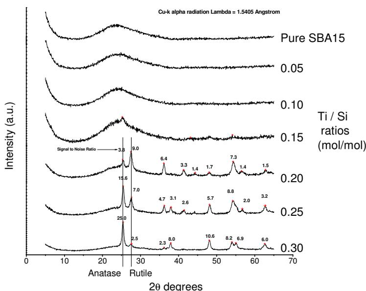
Figure 5. High-angle XRD patterns of TiO<sub>2</sub>-SBA-15 structures.
