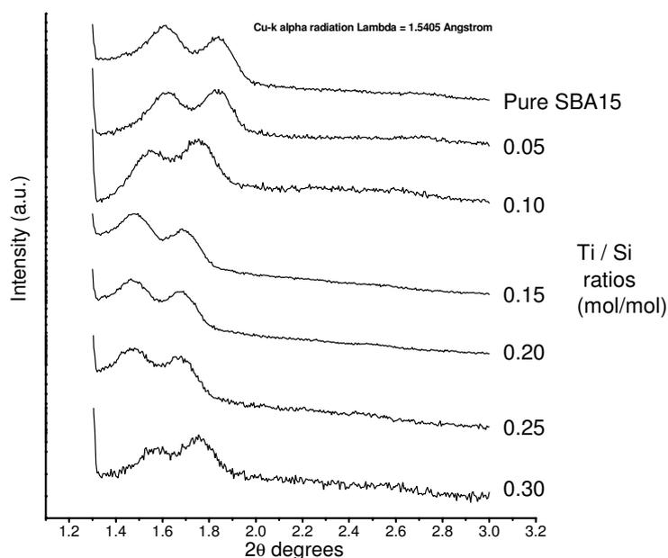
**Figure 4.** Low-angle XRD patterns of TiO<sub>2</sub>-SBA-15 structures.
