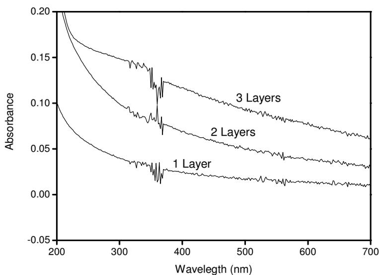
**Figure 2.** UV-VIS spectrum for TiO<sub>2</sub> film-coated ordinary glass dipped 1-3 times.
