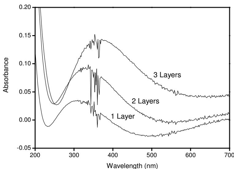
**Figure 3.** UV-VIS spectrum for TiO<sub>2</sub> film-coated ITO glass dipped 1-3 times.
