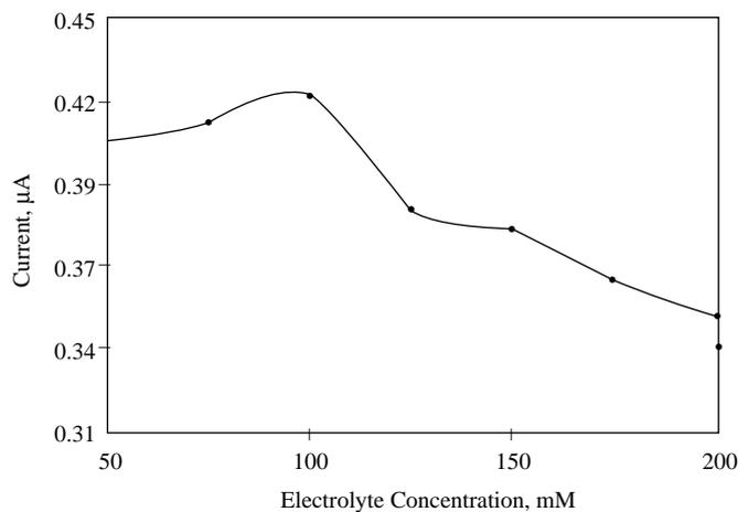
**Figure 5.** Effect of  $\text{KCl}$  concentration on the response.
