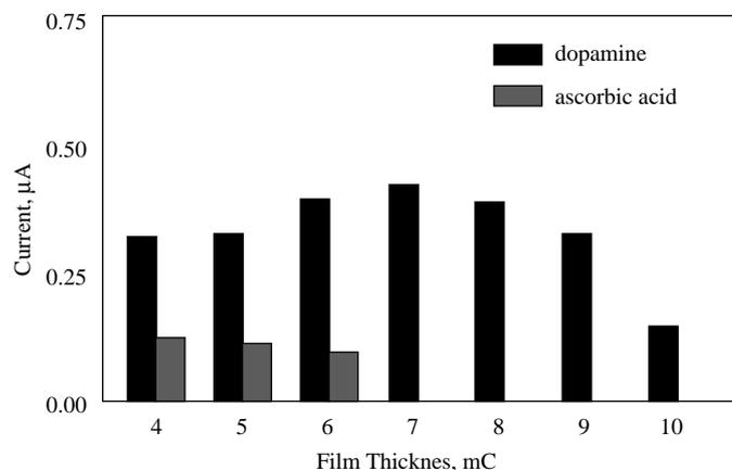
**Figure 2.** Effect of film thickness on the response.
