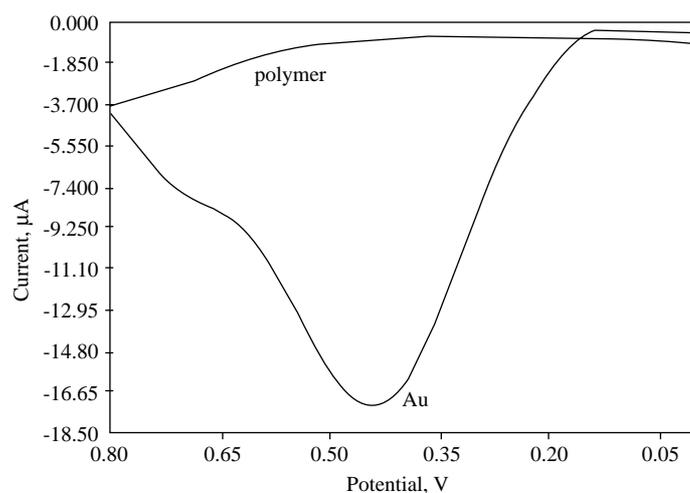
**Figure 6.** DPVs of 10 mM ascorbic acid at the bare and polymer electrodes.
