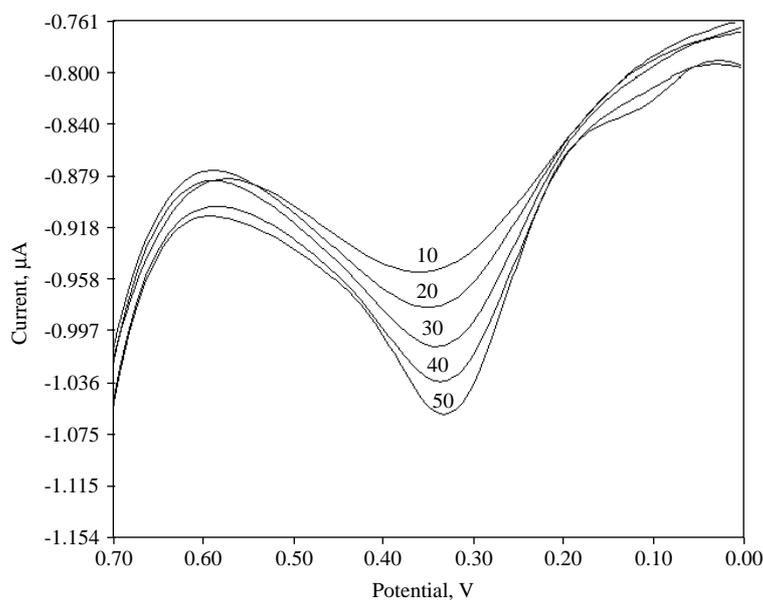
**Figure 7.** DPV of 10 mM ascorbic acid at various concentrations of dopamine (10-50 mM).
