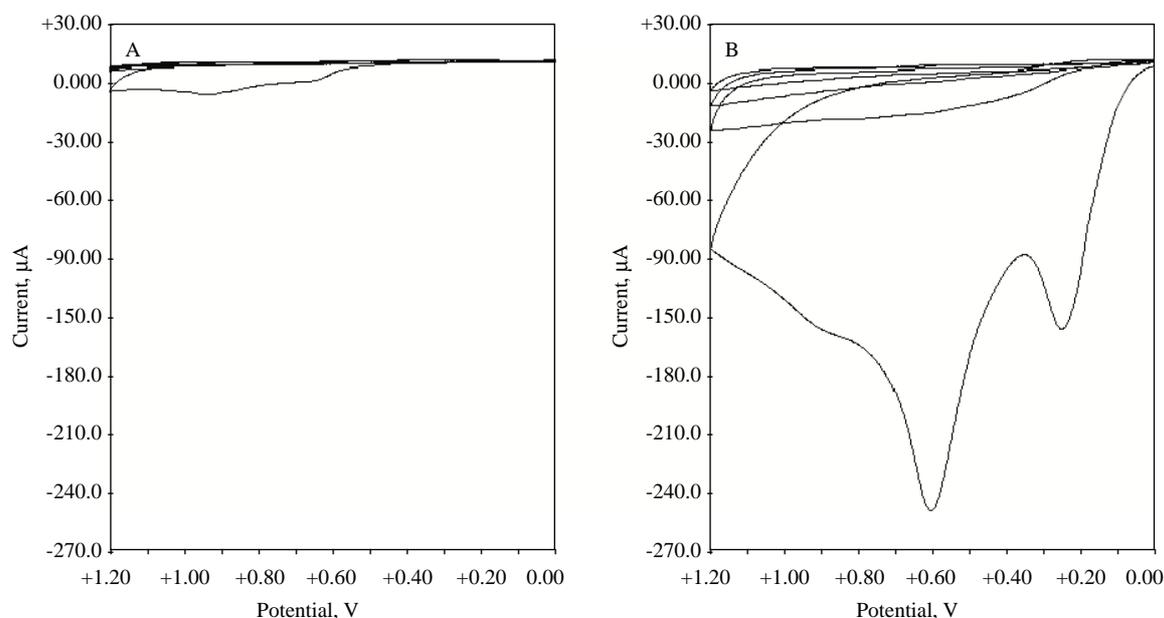
**Figure 1.** Cyclic voltammograms obtained with a bare Au electrode in 0.1 M KCl (A) and in 0.1 M KCl + 50 mM 1,4-diaminobenzene (B). Scan rate: 50 mV/s.
