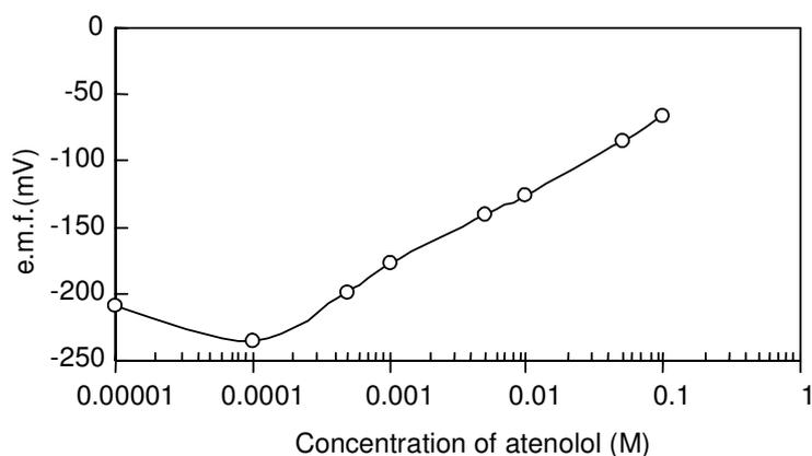
**Figure 2.** Calibration curve of atenolol selective electrode based on (A-TP) ionophore and DBPH plasticizer.
