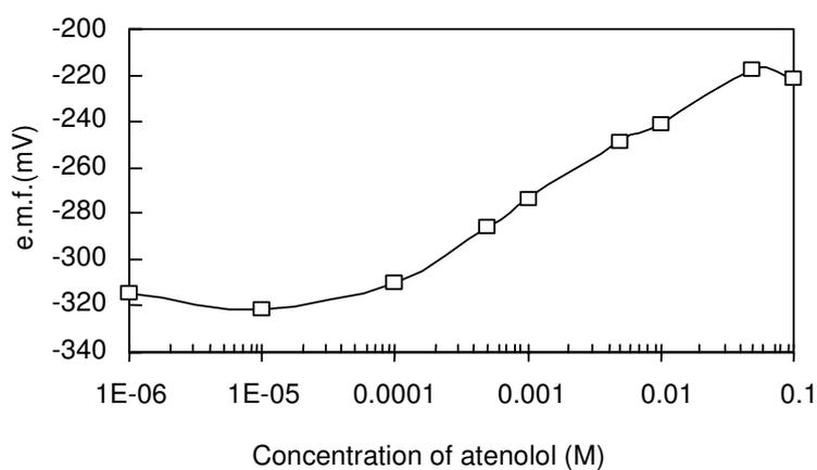
**Figure 1.** Calibration curve of atenolol selective electrode based on (A-TP) ionophore and DBP plasticizer.
