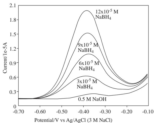
**Figure 4.** The square wave voltammograms of NaBH<sub>4</sub> on a Au electrode.
