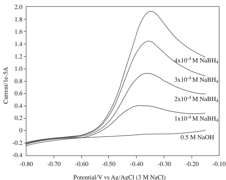
**Figure 1.** The cyclic voltammetric oxidation curve of  $\text{NaBH}_4$  on Au at different  $\text{BH}_4^-$  concentrations ( $v = 50 \text{ mV/s}$ ).
