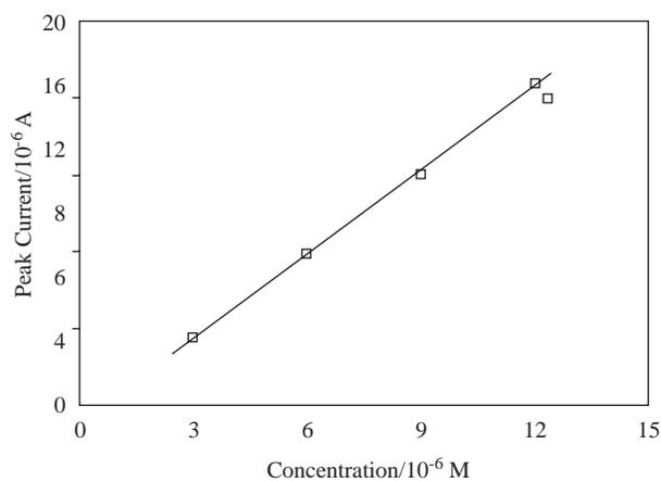
**Figure 5.** The changes in peak currents with NaBH<sub>4</sub> concentration on a Au electrode.
