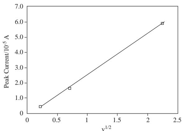
**Figure 3.**  $i_p - v^{1/2}$  plot of  $1.8 \times 10^{-5}$  M NaBH<sub>4</sub> on a Au electrode.
