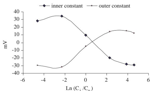
**Figure 1.** The changes in emf values versus  $\ln(C_i/C_o)$  with KCl solutions for inner surfaces and outer surfaces constant for periderm membranes.
