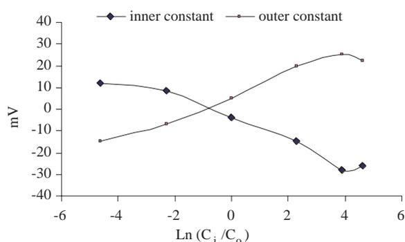
**Figure 2.** The changes of emf values versus  $\ln(C_i/C_o)$  with NaCl solutions for inner surfaces and outer surfaces constant for periderm membranes.
