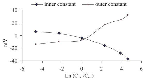
**Figure 4.** The changes of emf values versus  $\ln(C_i/C_o)$  with NaCl solutions for inner surfaces and outer surfaces constant for cuticular membranes.
