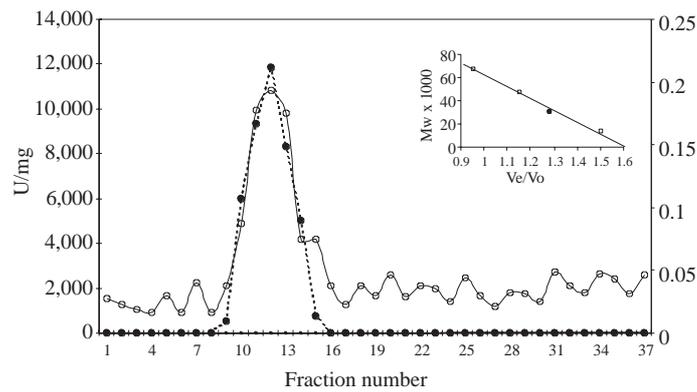
**Figure 3.** Gel chromatography on Sephadex G-100 of the collected chicken erythrocyte SOD fractions from the DEAE-cellulose column. (a) Absorbance at 280 nm (o—o), SOD activity fractions (● - - ●), and molecular weight calibration curve. (b) Protein markers (—o—), purified SOD (—●—).
