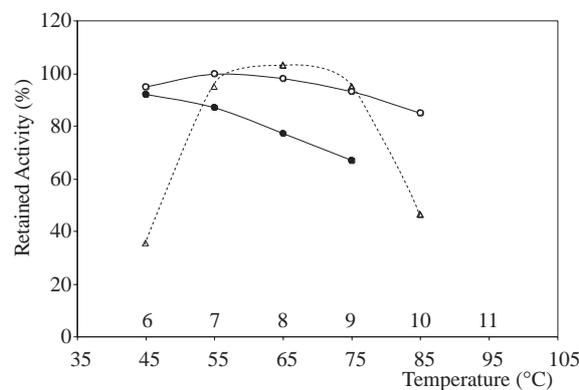
**Figure 5.** The effect of pH on the chicken erythrocyte CuZn-SOD activity at 25°C ( $\Delta$ - - $\Delta$ ); pH-stability variations for 2 h incubation at 25°C (o—o); temperature stability variations for 2 h incubation at pH 7.4 (●—●).
