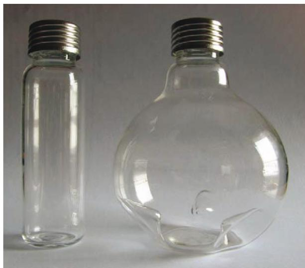
**Figure 1.** A standard headspace vial (Supelco, 20 mL) on the left and an artisan-made single-neck round-bottom flask (50 mL) on the right.
