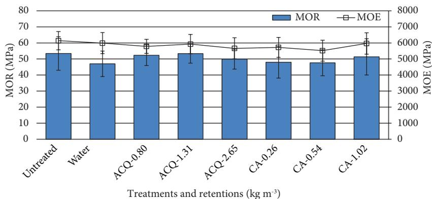
**Figure 1.** Effects of ACQ and CA treatments on mechanical properties (MOR and MOE) of posttreated SWP (mean of 10 replicates, error bars indicate ±standard deviations).
