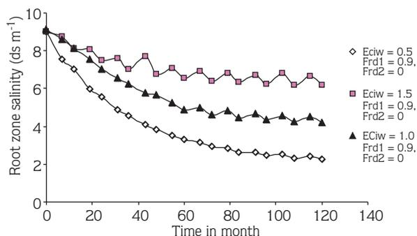
Figure 5. Effects of varying irrigation water salinities ( $EC_{iw}$ ) on the root zone salinity ( $EC_e$ ) in the controlled drainage conditions.
