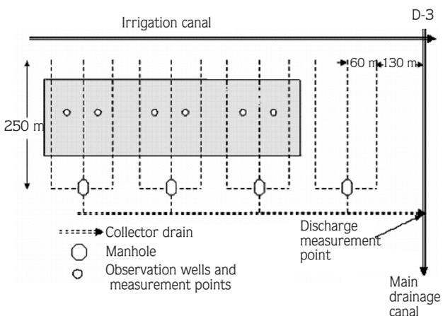
Figure 2. Layout of the experiment.
