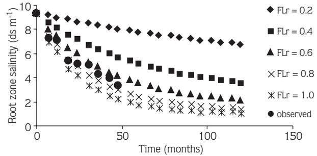
Figure 3. Calibration of root zone salinity and leaching efficiency in the test area.
