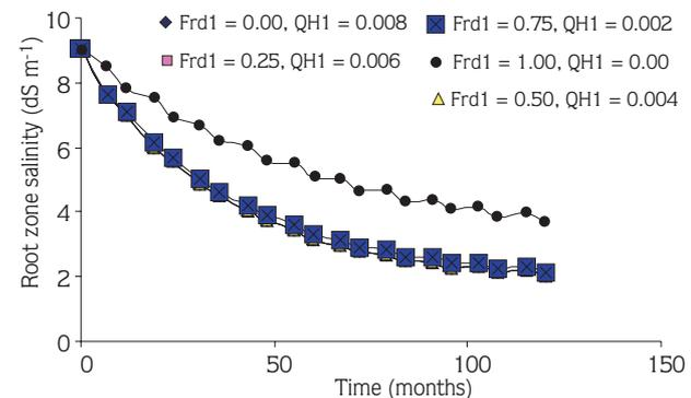
Figure 4. Effects of varying drainage control factors ( $F_{rd}$ ) on root zone salinity ( $EC_e$ ) for  $EC_{iw} = 0.470 \text{ dS m}^{-1}$ .
